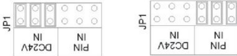
1. DC24V input jumper position
