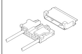
Board-to-wire crimping type connector with high withstanding voltage, used for power supply of large LCD (Liquid Crystal Display or Liquid Crystal Television) back light. Secure locking mechanism prevents from coming off housing when handling the wire harness.
