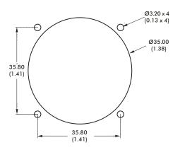
When mounted this way the panel acts as the bezel and no separate bezel is needed. M3 machine screws are recommended.
