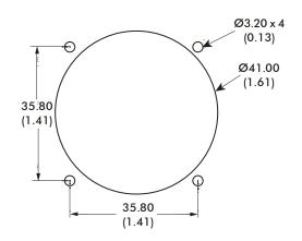
The joystick is dropped into the panel cut-out. The joystick and boot must be kept in place by bezel (option 6 & 7). For panel thickness of <3mm, M3 x 16 countersunk machine screws are recommended.
