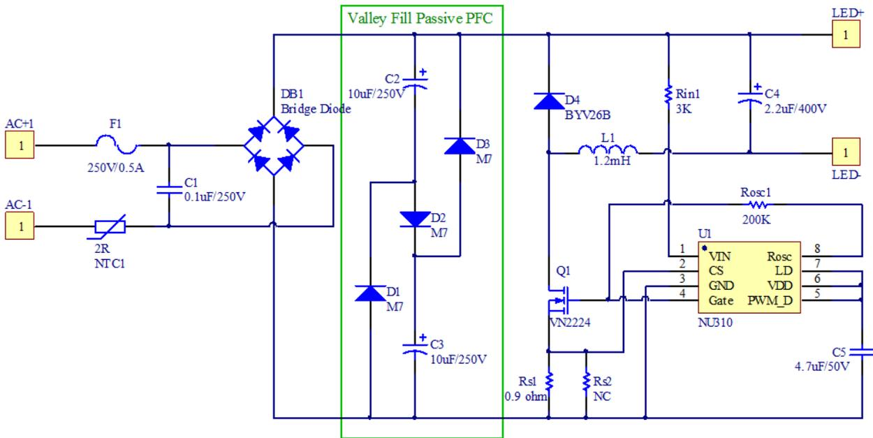
Figure 4: NU310 25V\_350mA Application Circuit
