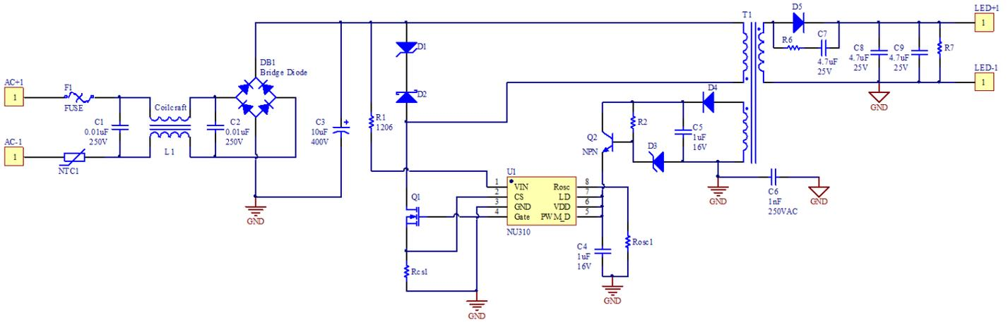
Figure 3: NUS310 75V\_220mA Application Circuit
