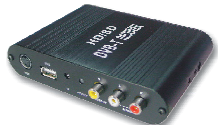
DTR-1307 Dimension: 132(L)x94(W)x27(H)mm Weight(Net): 290g
