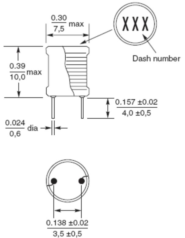
Dimensions are in  $\frac{\text{inches}}{\text{mm}}$
