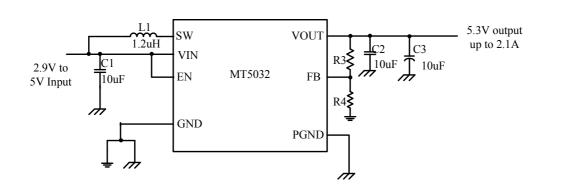
Figure 1. MT5032 Typical Application Circuit
