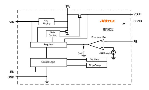
Figure 2. MT5032 Functional Block Diagram
