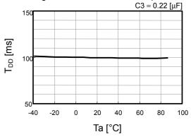
Overcurrent1 detection time vs. temperature
