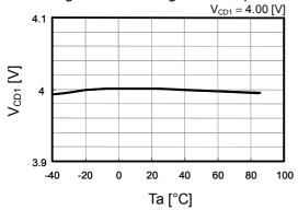
Overcharge release voltage2 vs. temperature
