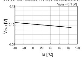
Overcurrent1 detection voltage vs. temperature
