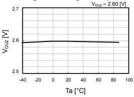
Overcurrent1 detection voltage vs. temperature
