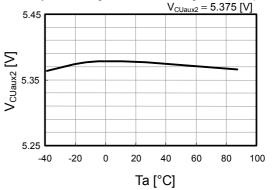
Overdischarge detection voltage1 vs. temperature
