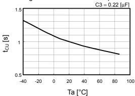
Overcharge detection1 time vs. temperature
