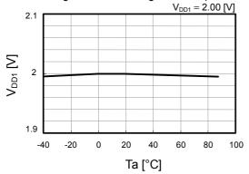
Overdischarge detection voltage2 vs. temperature
