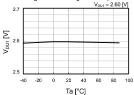
Overdischarge release voltage1 vs. temperature
