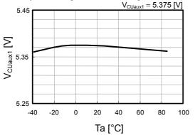
Auxiliary overcharge detection voltage2 vs. temperature
