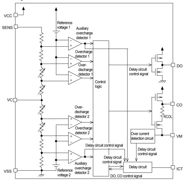
Remark Resistor (RCOL) is connected to the Nch transistor although CO pin serves as a CMOS output. For this, impedance becomes high when outputting "L" from CO pin. Refer to the "■ Electrical Characteristics" for the impedance value.
