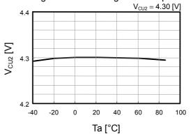
Overcharge release voltage1 vs. temperature
