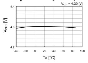
Overcharge detection voltage2 vs. temperature
