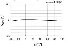
Auxiliary overcharge detection voltage1 vs. temperature
