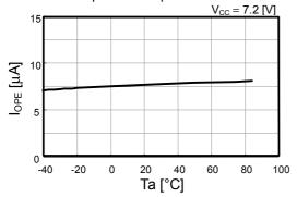
Current consumption vs. temperature in power-down mode
