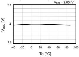
Overdischarge release voltage1 vs. temperature
