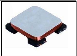
Keyless entry systems is a typical application for this coil, the isotropy is often sought in RF antenna. In transponder applications, this feature has been achieved by the combination of 3 single coils oriented in the 3 space axis with the aim of covering the maximum space orientation.
