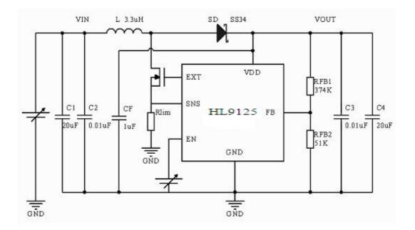
2) Power supply tied to VIN(VIN>2.8V)
