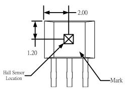
**Output Pin Assignment** (Top view)
