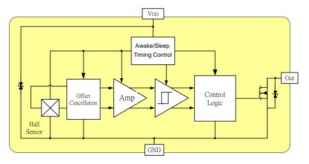
*Note:* Static sensitive device; please observe ESD precautions. Reverse  $V_{DD}$  protection is not included. For reverse voltage protection, a 100  $\Omega$  resistor in series with  $V_{DD}$  is recommended. *MH250, HBM* > ±4KV which is verified by third party lab.
