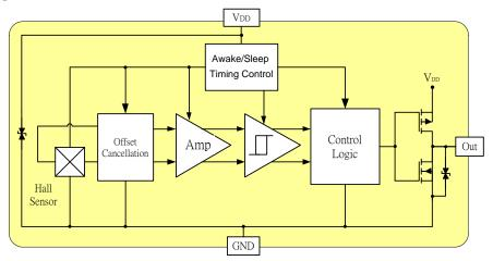
*Note*: Static sensitive device; please observe ESD precautions. Reverse  $V_{DD}$  protection is not included. For reverse voltage protection, a 100  $\Omega$  resistor in series with  $V_{DD}$  is recommended. *MH* 251, *HBM* > ±4KV which is verified by third party lab.
