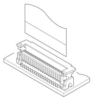
Vertical 0.3mm pitch ZIF type connector. This connector was mainly developed to connect FPC and subminiature digital products such as DVC, DSC, PDAs and so
