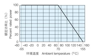
在环境温度70℃以上使用时,应按照左图负荷特性曲线,减小额定功率。 For resistors operated at an ambient temperature of 70°C or above, a power rating shall be derated in accordance with the left derating curve.
