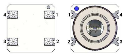
Figure 13: pin configuration
