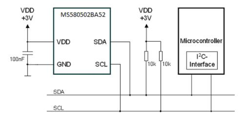
Figure 12: Typical application circuit with I<sup>2</sup>C protocol communication
