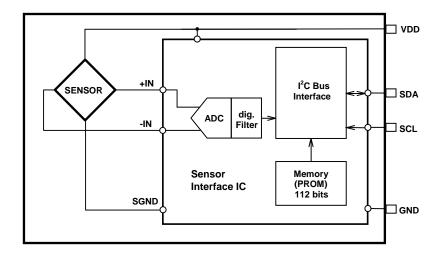
Figure 1: Block diagram of MS5805-02BA
