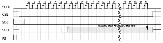
Figure 8: ADC Read sequence
