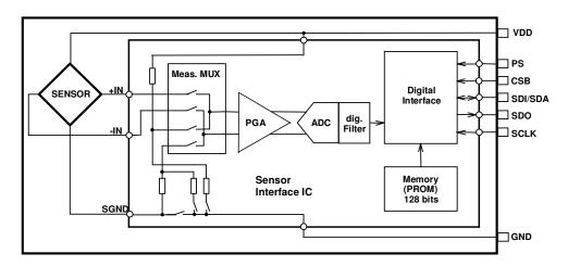
Figure 1: Block diagram of MS5803-01BA
