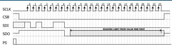
Figure 9: PROM Read sequence, address = 011 (Coefficient 3).
