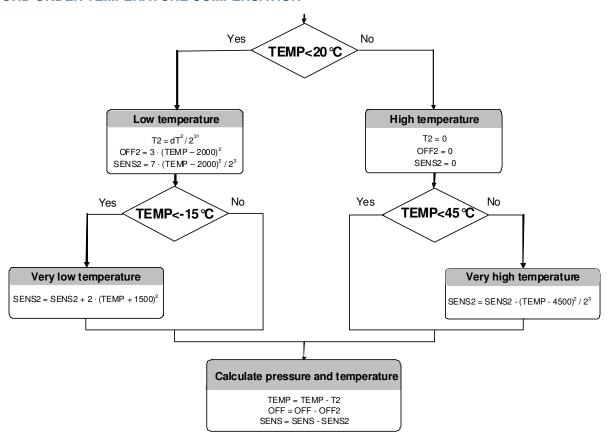
Figure 3: Flow chart for pressure and temperature to the optimum accuracy.
