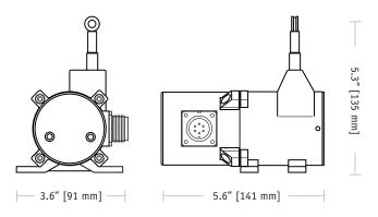
The PT8CN, using a high cycle plastic-hybrid potentiometer, communicates to your PLC via the CANbus SAE J1939 interface. Suitable for factory and harsh environment applications requiring linear position feedback in ranges up to 60".
