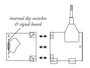
To gain access to the signal board, remove four Allen-Head Screws and remove rear cover.
