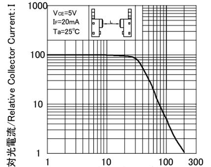
Distance between Emitter/Detector:  $L$  (mm)
