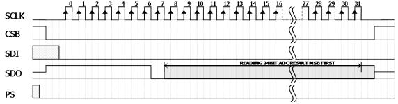
Figure 8: ADC Read sequence
