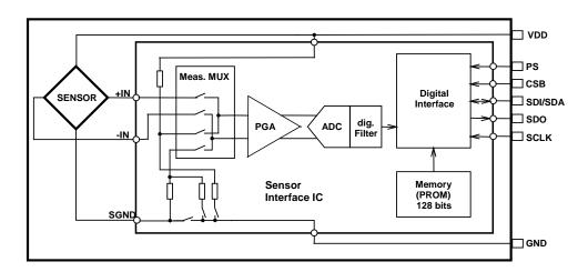
Figure 1: Block diagram of MS5803-05BA
