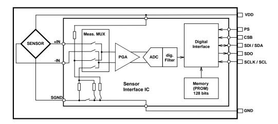
Figure 1: Block diagram of MS5803-14BA
