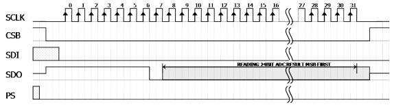
Figure 8: ADC Read sequence
