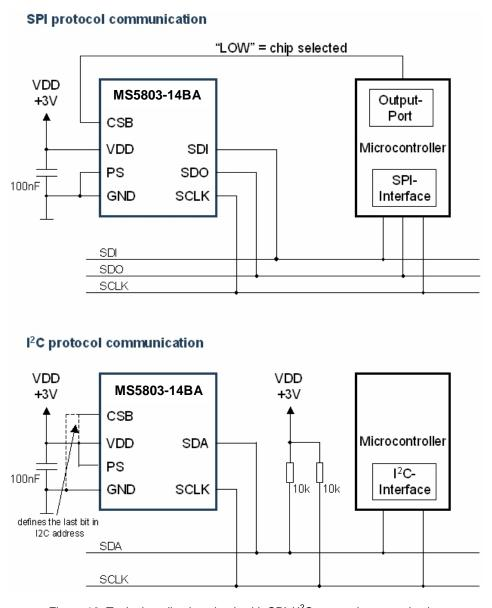
Figure 16: Typical application circuit with SPI / I<sup>2</sup>C protocol communication
