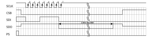
Figure 6: Reset command sequence SPI mode 3
