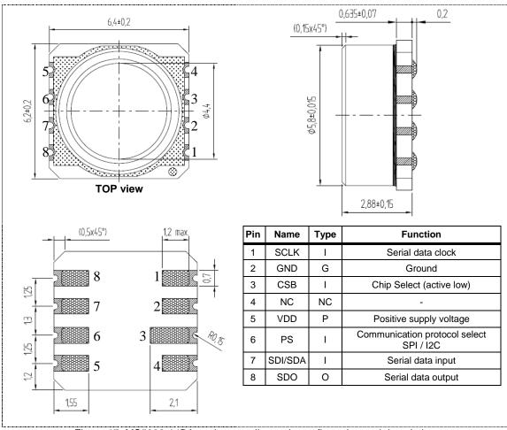
Figure 17: MS5803-14BA package outlines, pin configuration and description
