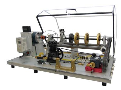
monitoring diagnosing and machinery faults before they irreversibly damage your machinery and cause breakdowns that threaten to undermine product quality, delivery and overall customer service. The success of any PdM program ultimately depends on how accurately and easily the vibration spectra, waveforms and phase relationships can be analyzed understood. Spectra and Quest's Machinery Fault Simulator Magnum (MFS-MG) is an innovative tool to study the signatures of common machinery faults without
