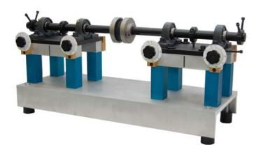
heads for alignment training. The innovative design makes it easy to extend the base to accommodate additional main modules for simulating multiple machine element trains. This can be done in both linear and perpendicular configurations. The SAT provides a range of benefits in developing an understanding of alignment problems.
