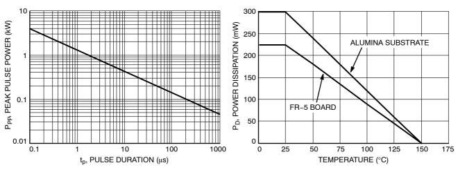
Figure 1. Non-Repetitive Peak Pulse Power versus Pulse Time
