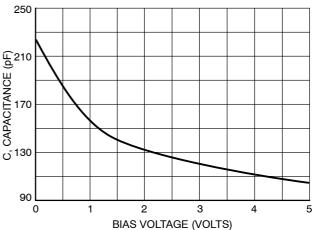
Figure 4. Typical Diode Capacitance (SM05)
