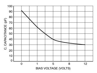
Figure 5. Typical Diode Capacitance (SM12)
