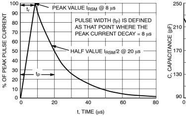
Figure 3.  $8\times20~\mu s$  Pulse Waveform
