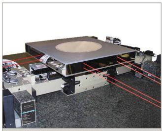
Multi-axis interferometer feedback is available to control Xand Y position, as well as Y-axis yaw. Use of a remote detector allows one laser source to be used for multiple axes.
