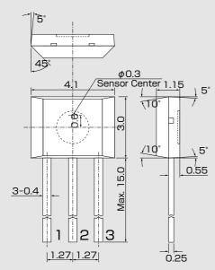
Note) The sensor center is located within the  $\phi$ 0.3mm circle.
