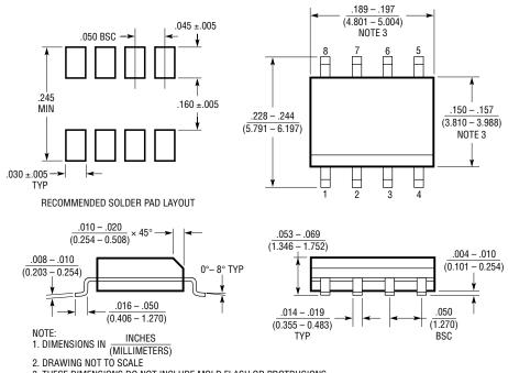
3. THESE DIMENSIONS DO NOT INCLUDE MOLD FLASH OR PROTRUSIONS. MOLD FLASH OR PROTRUSIONS SHALL NOT EXCEED .006" (0.15mm)
