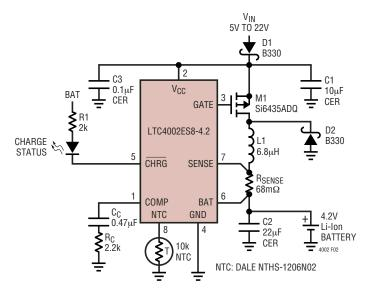
Figure 2. 1.5A Single Cell Li-Ion Battery Charger
