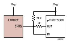
Figure 1. Microprocessor Interface
