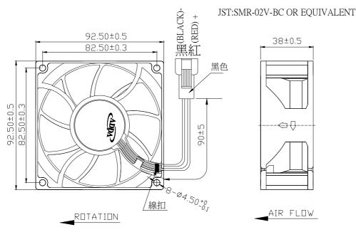
LEAD WIRES : UL 1007, AWG24 , L =  $90\pm 5$  mm Red = positive ; Black = negative.
