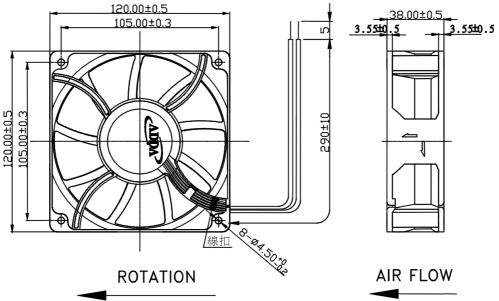
LEAD WIRES: UL 1007, AWG24, L = 290±10 mm
