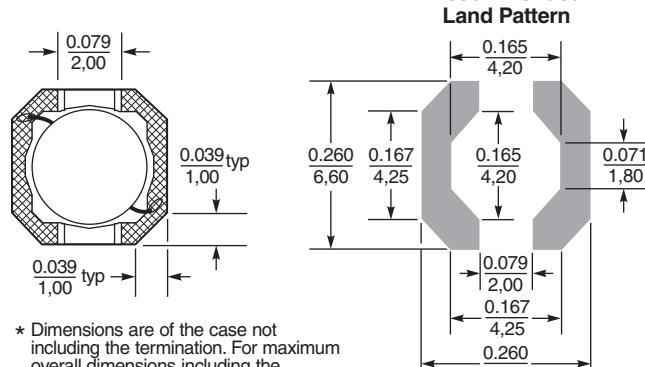
\* Dimensions are of the case not including the termination. For maximum overall dimensions including the termination, add 0.005 in / 0,13 mm.
