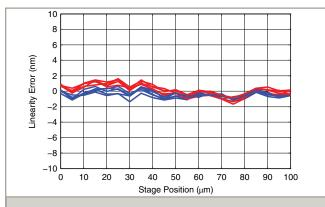
QNP-40-100XY upper-axis linearity error plot measured with a laser interferometer over multiple bidirectional runs. The linearity measured is <0.002%. All sizes of the QNP stage series exhibit exceptional linearity and repeatability.
