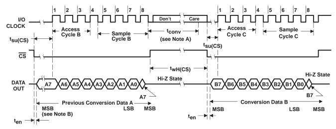
NOTES: A. The conversion cycle, which requires 36 internal system clock periods (17 µs maximum), is initiated with the eighth I/O clock pulse trailing edge after CS goes low for the channel whose address exists in memory at the time.
