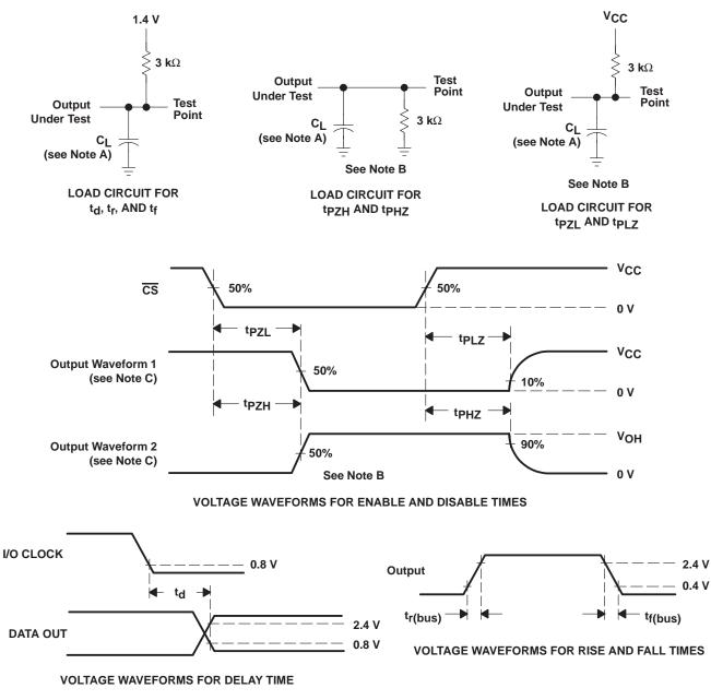
NOTES: A. CL = 50 pF for TLC548 and 100 pF for TLC549; CL includes jig capacitance.
