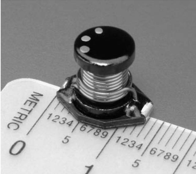
These surface mount power inductors provide excellent current carrying capabilities in a small footprint component — up to 3.5 Arms with an 8 Adc saturation current rating for a 10  $\mu\text{H}$  part.
