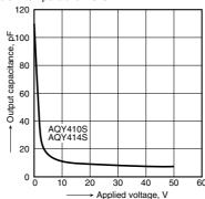
12-(2). Output capacitance vs. applied voltage characteristics
