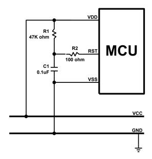
This is the basic reset circuit, and only includes R1 and C1. The RC circuit operation makes a slow rising signal into reset pin as power up. The reset signal is slower than VDD power up timing and system occur to a power on signal from the timing difference.
