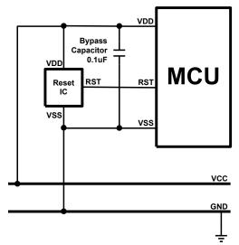
The external reset circuit is also to use external reset IC to enhance MCU reset performance. This is a high cost and good effect solution. By different application and system requirement to select suitable reset IC. The reset circuit can improve all power variation.
