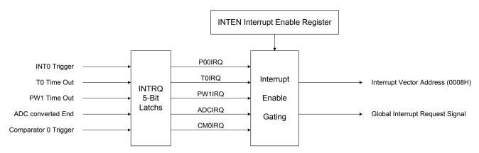
Note: The GIE bit must enable during all interrupt operation.
