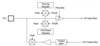
• Bi-direction shared pin structure with specific digital output function (e.g. PWM, .....):
