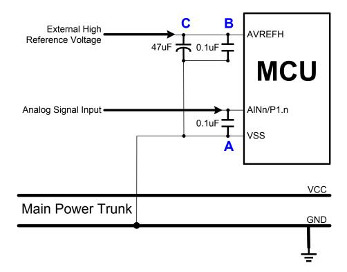
The analog signal is inputted to ADC input pin "AlNn/P1.n". The ADC input signal must be through a 0.1uF capacitor "A". The 0.1uF capacitor is set between ADC input pin and VSS pin, and must be on the side of the ADC input pin as possible. Don't connect the capacitor's ground pin to ground plain directly, and must be through VSS pin. The capacitor can reduce the power noise effective coupled with the analog signal.
