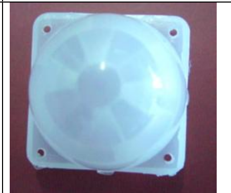
8002-1,边长:24mm,高:19.6 焦距:11mm,角度:100,距离:5m,
