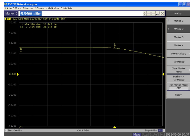
Figure 4 Typical P1dB 3 GHz measurement result
