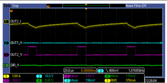
Figure 8. 50% Duty Cycle, Reverse Direction
