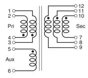
The primary windings and the secondary windings are to be connected in parallel on the PC board.
