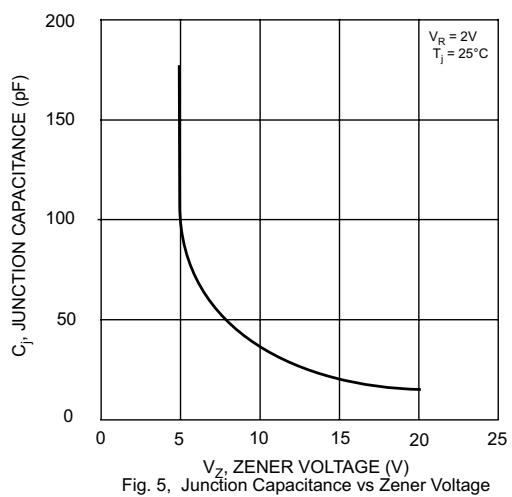
Fig. 5, Junction Capacitance vs Zener Voltage
