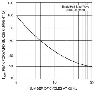
Fig. 3 Forward Surge Current Derating Curve
