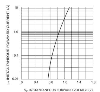
Fig. 2 Typical Forward Characteristics
