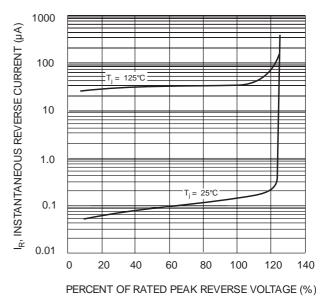
Fig. 4 Typical Reverse Characteristics
