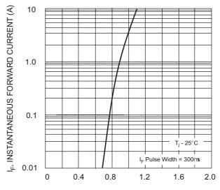
$V_{\rm F}$ , INSTANTANEOUS FORWARD VOLTAGE (V) Fig. 2 Typical Forward Characteristics
