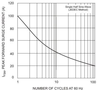
Fig. 3 Forward Surge Current Derating Curve
