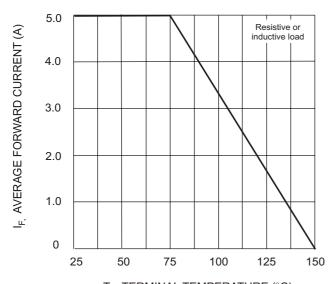
T<sub>T</sub>, TERMINAL TEMPERATURE (°C) Fig. 1 Forward Current Derating Curve
