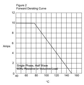
Average Forward Rectified Current - Amperes versus Case Temperature -  $^{\circ}\text{C}$
